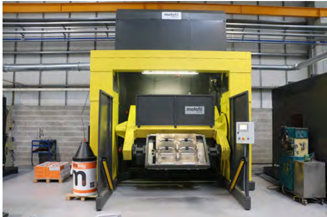
Mlean Ferris Wheel Welding System Load capacity from 300 to 1000 Kg
