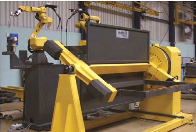
Ferris Wheel Welding System Load capacity from 300 to 1000 Kg
