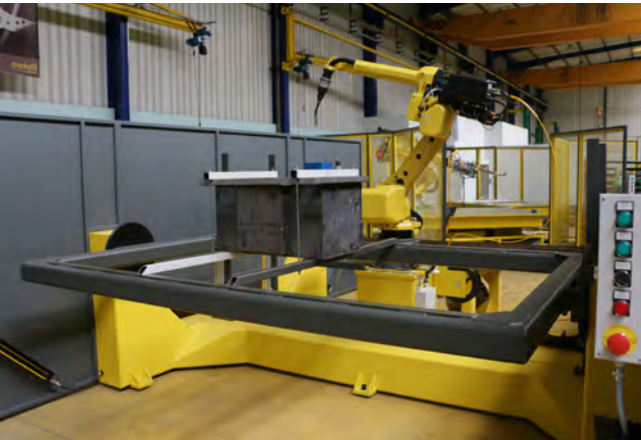
Monoblock Front/Back Configuration Load capacity from 300 to 2000 Kg
