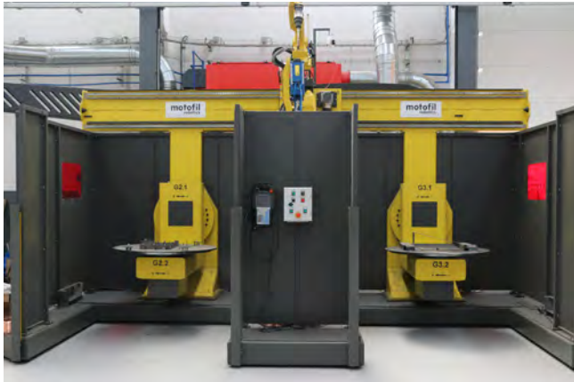
Classic Double Sky-Hook Welding System Load capacity from 300 to 1500 Kg
