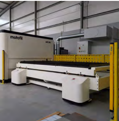
MFL - Fiber Laser Cutting Machine (with the option of a automatic loading and unloading system)
