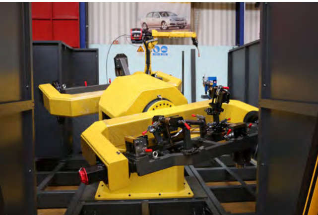
5-Axis H-Table Welding System Load capacity from 300 to 600 Kg
