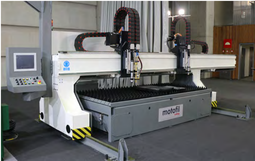
DRAGOm - Multiprocess System (Plasma Cutting, Oxyfuel and Mechanical Drilling)
