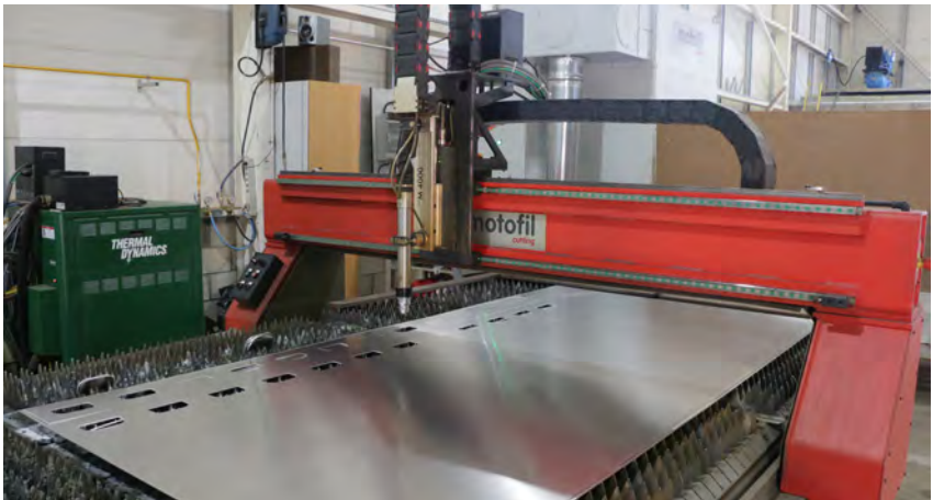
FELINE - Plasma Cutting Machine Cuts different types of metal with a maximum thickness of 25mm
