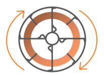
Verify **cast and hélix** removing, without any pressure on the wire, 4 - 5 loops from the spool and place it on the floor:
